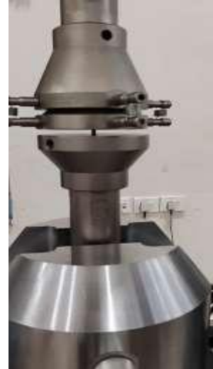
Figure 7 Compressive strength was determined at a-cross head speed of 0.5mm/min in universal testing machine
